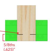
Please use only enough clamping force to hold the wood block in the jig. Too much force can skew the wood or with enough pressure, flex the jig resulting in misaligned axle holes.
