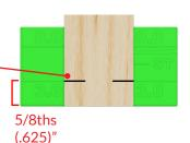
Please use only enough clamping force to hold the wood block in the jig. Too much force can skew the wood or with enough pressure, flex the jig resulting in misaligned axle holes.
