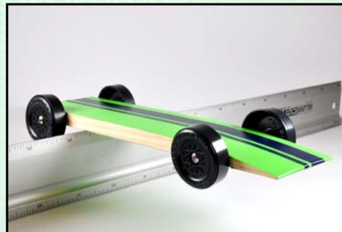
A ruler or other straight edge makes a good tool to help fine-tune the COG.
