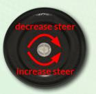
If you do not have access to a track to tune on, a good car setup would be 16-17 grams (0.56-0.60 oz) on the front wheel and 4-5 inches of steer!
