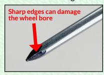
down, and then finish with 400 and 800-grit sandpaper. The <u>axle prep kit</u> contains a special tool to insert the axle into a drill. Otherwise, you'll need to complete this step by hand. There is no need to go with the higher grit
