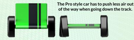
The other main advantage of a thin car is it helps to maximize potential energy. The slender bodies are much lighter than more traditional designs. By removing most of the wood weight from the car body, the racer can **place the weight in the optimal location** for maximum speed. Weight placement is discussed in more detail in the <u>Weighting chapter</u>.
