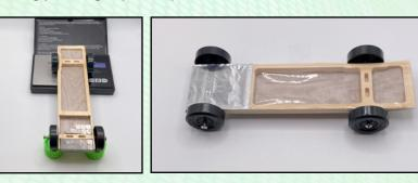
Insert the wheels and axles all the way. For rail riding setups, you will want the right front axle head of the bent axle to point downward.
