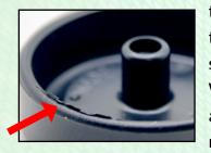
the edge of the wheel while spinning it with the drill. **Do not over-sand**; you want to sand just enough to remove the flashing. With modified wheels, you'll want to sand off any burs from the cutting process but don't round over the edge. Next, use a wet paper
