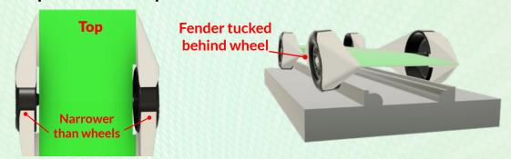
Failure to properly shape the fenders will **result in a significant increase in drag/friction**, negating the benefit of the fenders. In many cases, a poorly done fender car will be **SLOWER** than a similar car with no fenders.
