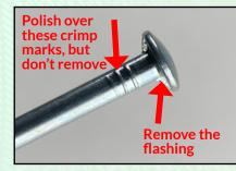
Removing the crimp marks on the axle shaft will significantly reduce the diameter of the axle. Crimp mark removal gives the wheel more room to move on the axle, making it more likely the wheel will vibrate, causing the car to wiggle. An unstable, wiggling car is slow.
