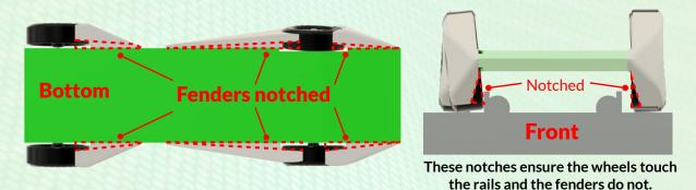
2. <u>Forward profile</u> - The fenders should be shaped to cover the wheels' forward profile. Some clearance on the bottom and top is ok.
