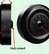
Modified wheels are lighter and have reduced contact points with the axle, car body, and track. As a result, these wheels decrease friction, drag, and rolling inertia, resulting in a much faster car!
