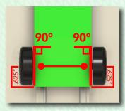
The rear wheels must be parallel to each other and the car body. Additionally, the wheels must be located directly across from one another. Finally, if rules do not prohibit, the rear axle holes should be placed 5/8ths (0.625) of an inch from the car's rear. Moving
