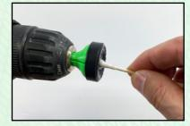
spinning the wheel, use medium pressure to polish the outer hub. If using stock wheels from the kit, you'll want to concentrate on the outer step. Polish for 1-2 minutes adding polish every 30 seconds. Use a wet
