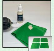
microfiber or cotton cloth. Polish the shaft and underneath the axle head for 60 seconds each. SUP BE CAREFUL; the cloth can entangle the axle and pull fingers in with it. Cutting the microfiber or cotton cloth into smaller pieces helps prevent this.
