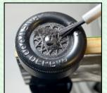
way under the axle head and into the wheel bore. Turn the car so the wheel faces the ground and spin the wheel several times. Repeat this process with the inner hub. Apply graphite and tap the wheel to spread the graphite into the inner hub and between the wheel and the car body. Turn the car so the wheel faces up and spin it several times. A soft bristle paintbrush works well to push graphite under the axle head and onto the inner hub. Add more graphite and repeat.
