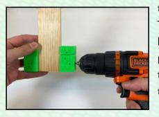
the <u>Alignment</u> chapter of this book. There are <u>tools</u> available that have been designed specifically for this purpose. The car body fits into the tool, and the axle holes are drilled in the correct positions.
