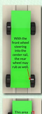
removed a precise amount The front wheel steers into the rail to stabilize the car. A stable car is much faster than one that wiggles. However, if not addressed, the rear wheel on the same side as the steer wheel will also rub the center rail creating additional friction that yields no benefit.
